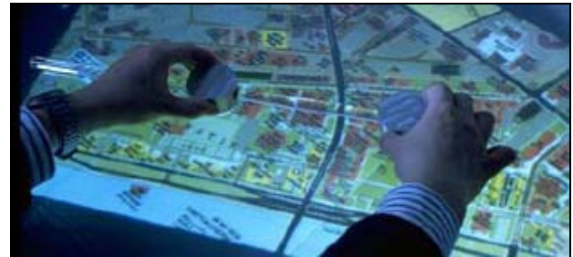
Figure 1. Tangible Media Group's metaDesk allows how users manipulate and display information simultaneously, demoed at the Media lab in 1997.
