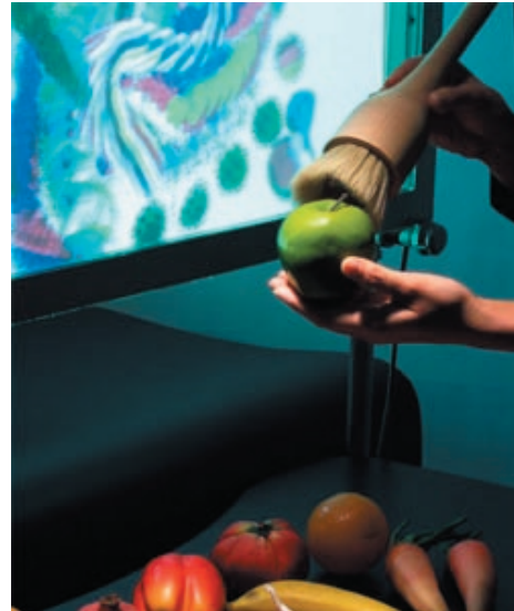
Figure 3. With IO Brush, children can paint with the color and movement of any object.
