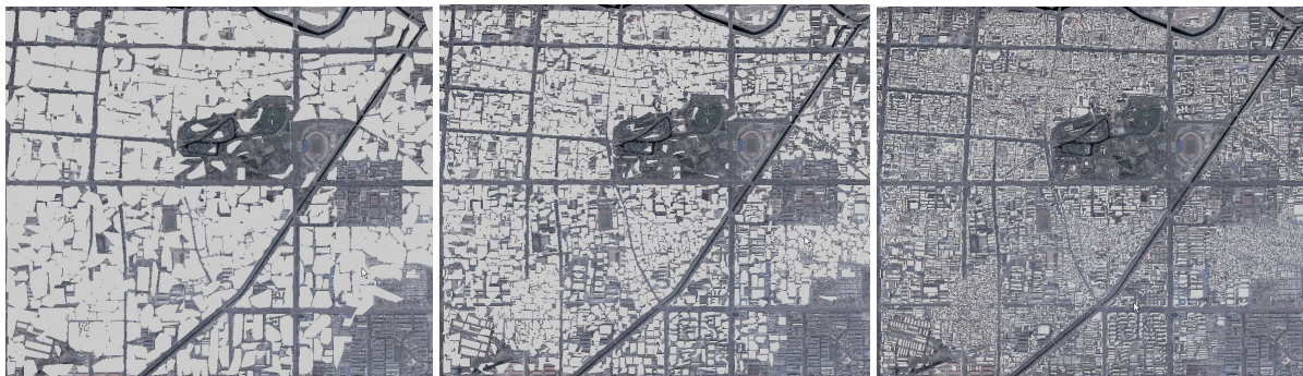
Figure 14. Finding elements of urban legibility. To correctly identify the elements of urban legibility and hierarchically categorize them from the most to the least important, we overlay different levels of detail of the urban model over GIS data that contain information on roads, districts, etc. The images from left to right show the urban model in decreasing LoD. The coarsest level of the model retains the most significant elements in the city such as the waterway that cuts through the city diagonally, the park in the center of the city, and the main road that runs east-west through the city; whereas the finest level of detail contain much finer elements that are only significant in a localized way.
