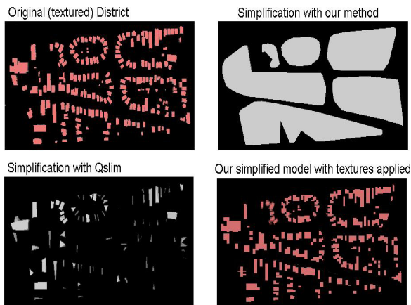
Figure 8. Comparison of our method (right) to original data (top left) and to a well known simplification method (Qslim [Gar197], bottom left). Both methods have the same number of polygons, but Qslim loses all sense of the original model. After texturing, our greatly simplified model (bottom right) retains the features of the original model.
