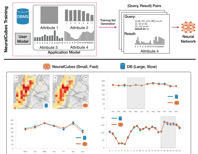
Fig. 1. NeuralCubes frames approximate query processing over a database as a neural network, one that takes a query as input, e.g. selection of a temporal interval, and maps it to an aggregation result as output, e.g. a count of the number of records, enabling real-time visual exploration for large-scale data. In the figures above, the blue lines represent visualizations generated with data from the database and the orange lines are generated using NeuralCubes. Note that the two are nearly indistinguishable, but NeuralCubes uses only a fraction of the memory footprint as the database.
