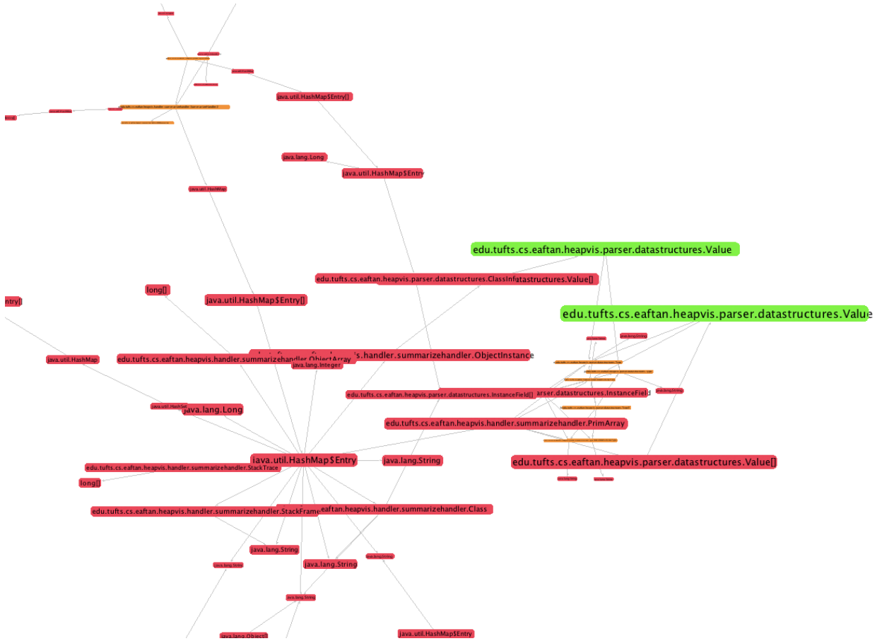
Figure 15: A Heapviz visualization of an early version of its own heap analyzer component. In the upper right, we see two large nodes of type Value (shown in green) that represent over 2 MB of memory usage.
