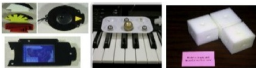
Fig. 1. TVE [Zigelbaum et al. 2007] (left): a TUI for collaborative video editing, implemented with communicating handheld computers. Marble Track Audio Manipulator [Bean et al. 2008] (center): an augmented toy for collaborative music authoring, implemented with an IPAC controller. Smart Blocks [Girouard et al. 2007] (right): computational manipulatives for learning basic geometrical concepts, implemented with RFID.
