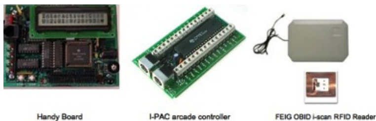
Fig. 23. TUI implementation technologies supported by our proof-of-concept TUIMS prototype.
