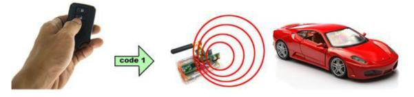
Figure 9. The RollJam, detecting a signal, jams the vehicle's frequency. The code is intercepted and stored [7].
