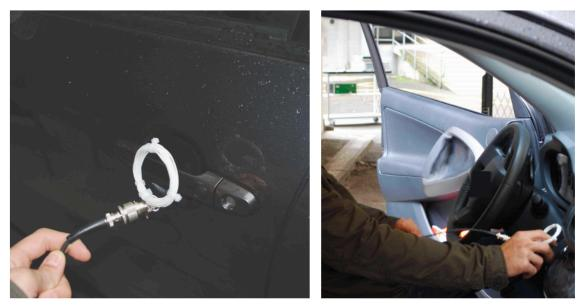
(a) Loop antenna placed next to the door handle.
