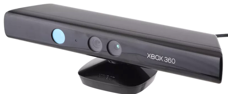
Microsoft Kinect RGB-D camera
