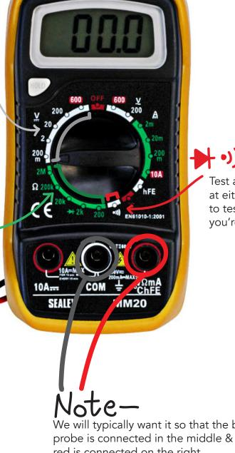
>>>) Continuity Test a connection. Put probes
