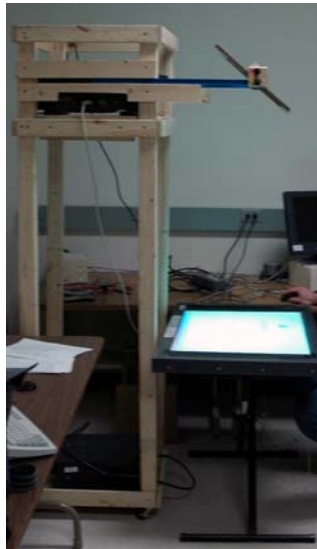
Figure 6: The study environment, showing the DiamondTouch™ screen with image projected from above.
