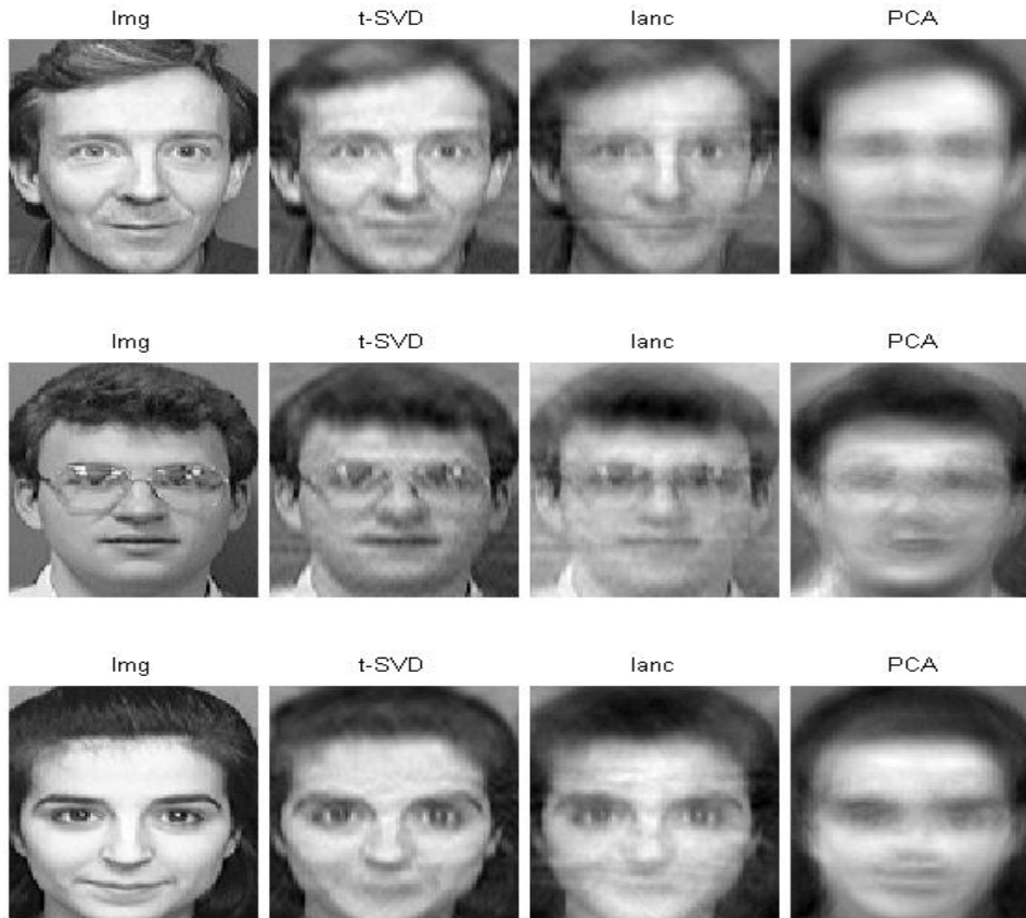
FIG. 7.3. Reconstructions of certain views of individuals in the AT&T database. Left is using 20 columns of the t -SVD U matrix; middle is using 20 columns of the estimates of U via our bidiagonalization; Right is using 20 terms of traditional PCA. Note the similarity between the leftmost pair of reconstructions, and their superiority over the more traditional PCA approach.
