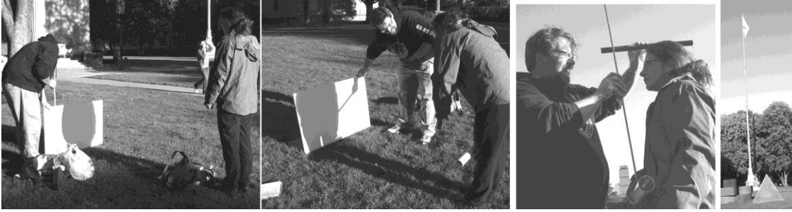
Figure 5. Marco measures the height of the shadow of Emanuela’s head [left] and hips [left middle] on a white board before measuring her head’s height [right middle]. Right: The flagpole’s shadow falls on upright trees.
