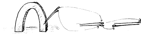
Fig. 4. Two needle tips are touched to the same horseshoe side, and laid with tips matching. They immediately swing around; one needle's eye now matches the other's tip.
