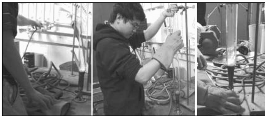
Figure 5. Left – Mingwei adjusts the valve to the burner's gas line. Middle – Mingwei lowers the tube over the burner (Photo Martin Demaine). Right – Mingwei adjusts the air flow into the burner.
