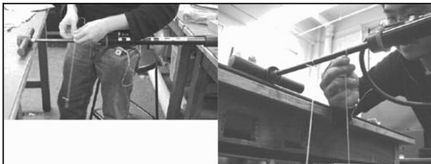
Figure 1. Left – Mingwei uses a bike pump's shaft as the support for a pendulum's string. Right – Mingwei adjusts the length of two pendulum strings.
