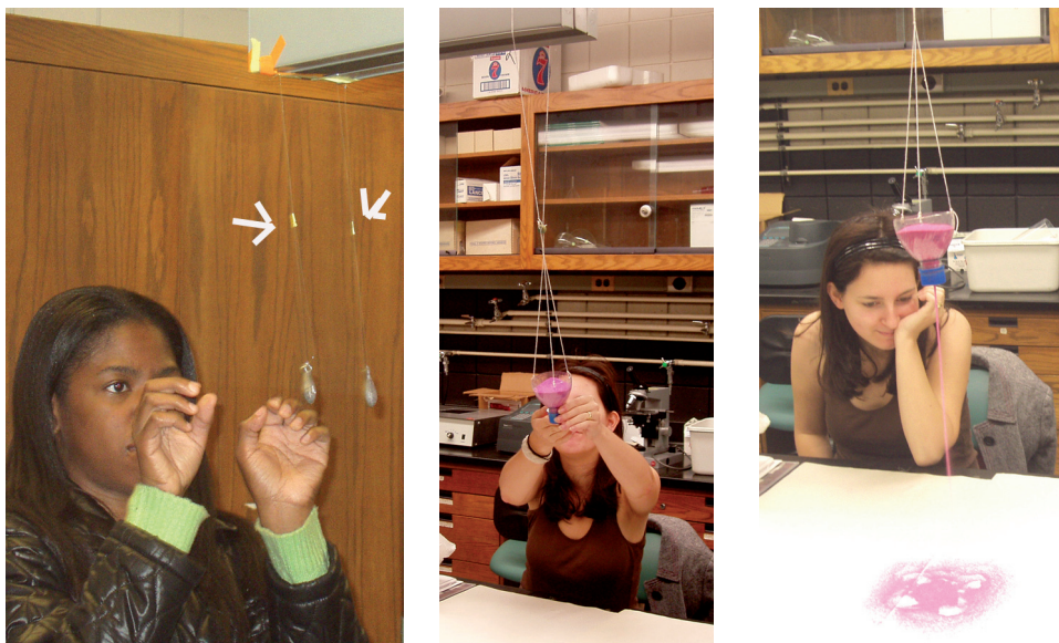
Figure 8. Left: Lucienne releases two pendulums together. The pendulums are interlinked by a horizontal thread (not visible) that is taped to their two vertical strings near the arrow heads. Middle: Samantha releases a pendulum supported by two long strings that cross midway and support a transparent cup of pink sand as the weight. Right: Samantha watches pink sand leak out of the swinging pendulum cup, producing overlapping figure eight patterns on the white paper below.
