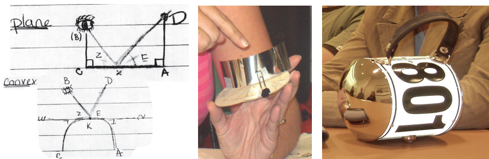
Figure 7. Left: Jennimae's diagrams redoing Euclid's argument for equal angle reflection in flat and convex mirrors. In both, her eye is depicted at point B , looking at point K on the mirror at the reflection of the object D . Angle Z is equal to angle E in both the case of the flat mirror CKA (top) and the curved mirror CKA (bottom, Cronan, 2005) Middle: Jennimae's replication of Ptolemy's apparatus has a mylar mirror sheet bent convex mounted on a circular disc like Ptolemy's, and uses a paperclip as a sighting aid. Right: Jennimae's mirror purse is cylindrical shaped, having the numbers 801 printed around its cylinder sides, and convex mirrors making up either end.
