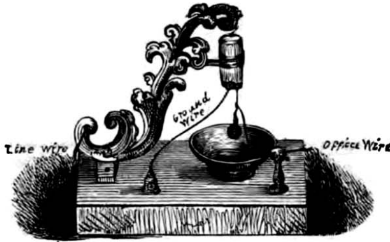
Figure 9.5. In this lightning arrester by Royal House, the signal wire on the left attaches to the ornamental brass support and enters a fine wire that passes through a hole in the cylindrical weight and connects to the office equipment. The fine wire supports the weight by a silk thread so that when high voltages pass on the fine wire, the wire breaks and the weight falls and transmits the discharge to ground. Turnbull, Electro-Magnetic Telegraph , 188.
