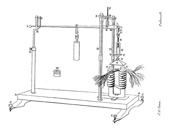
Figure 6. Hearder's ``magnetometer'' is wound with 24 wires which may be connected in parallel or series (Hearder 1844).
