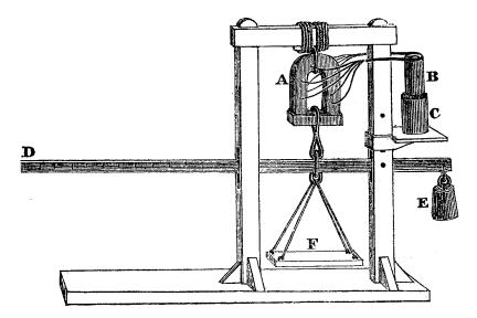
Figure 1. By adding weights to tray F, the maximal load capacity of Henry's electromagnet, A, could be determined. The galvanic plates, B, are depicted out of the cup, C, containing the acid. From (Henry 1831a).
