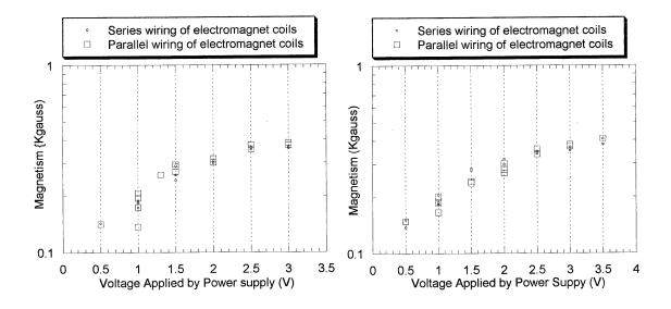
Figure 5. Readings (in kilogauss) of the magnetic field produced by a nail electromagnet activated by a power supply operating at fixed values of voltage (but variable current). For this very low resistance supply, the nail's electromagnetism is nearly the same under series (dot) and parallel (box) connections of the coils.
