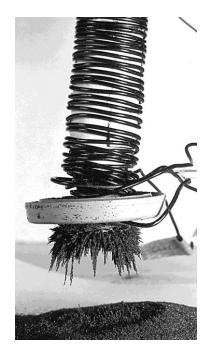
Figure 3. My electromagnet: a long nail that lifts magnetite sand from a pile when its coiled wires are connected to D cells. Photo by Joe Peidle.
