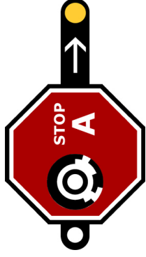
Figure 5: A SpotCode is printed on every statement of the language. This code allows us to determine the position, size, orientation, and type of individual statement in a program.
