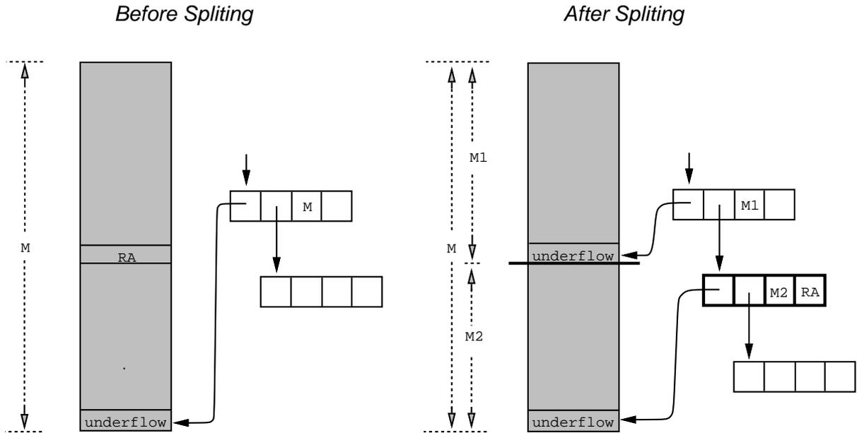
**Figure 7.** Large stack segments must be split before being reinstated. A splitting point is found by walking the stack to find the frame that gives the largest value for  $M1$  without exceeding the predetermined limit on copying. The return address at the splitting point is stored in a new stack record and the address of an underflow handler is stored in its place.
