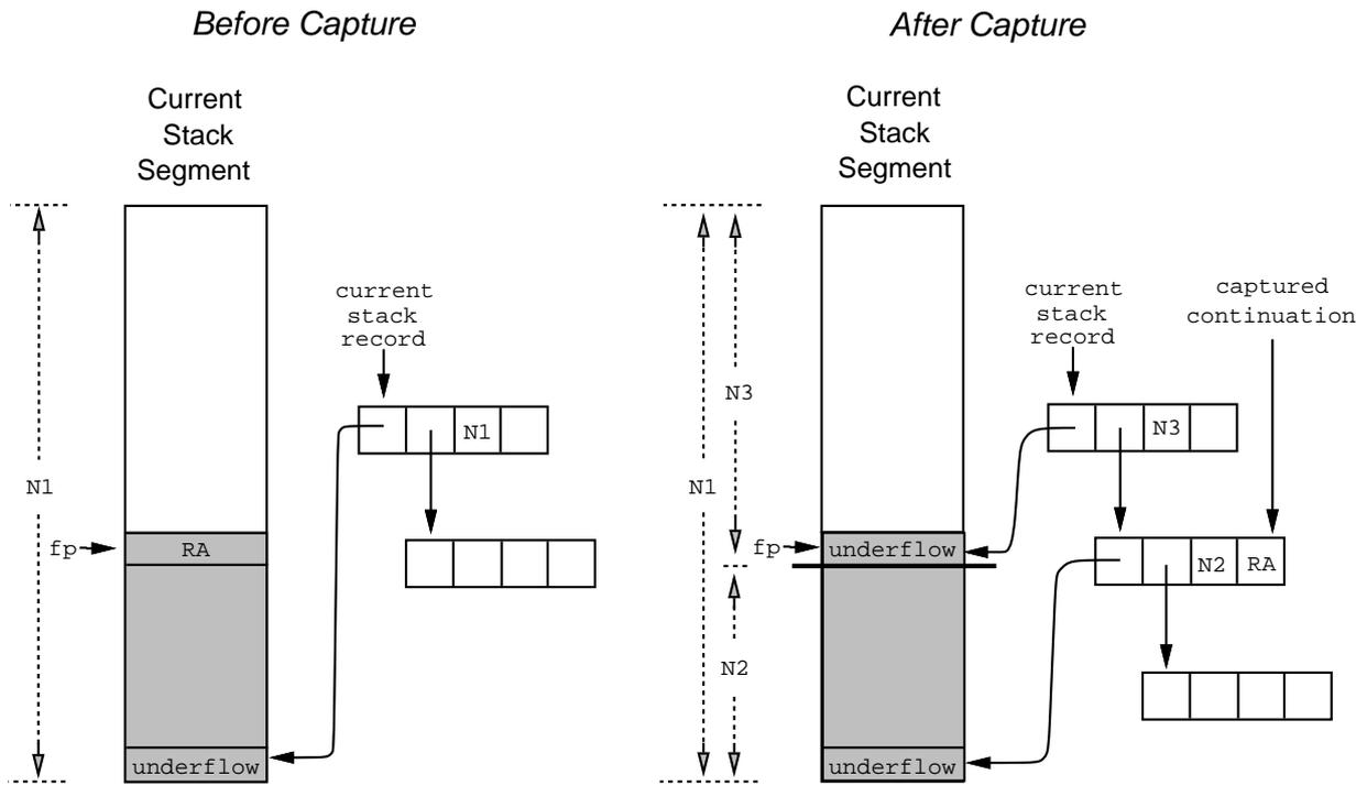
**Figure 5.** Capturing a continuation is a constant-time operation with the segmented stack model. The current stack segment is divided into two segments at the top frame. The bottom segment is the stack segment for the captured continuation, and the top segment becomes the current stack segment.
