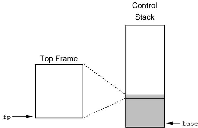
**Figure 2.** The traditional stack model provides the least expensive frame linkage. Since frames are physically adjacent, frame links can be maintained by simple register adjustments. However, since continuation operations require time proportional to the size of the active portion of the stack, the amount of time required is effectively unbounded.
