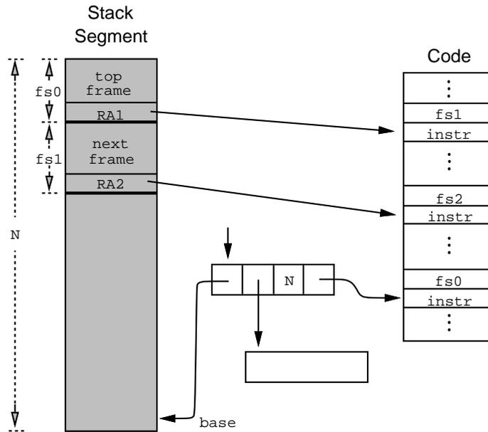
**Figure 4.** Walking backwards through a stack segment is straightforward. The return address field of a continuation stack record points to an instruction in the code stream, which is preceded by a data word containing the frame size. This frame size is used to find the base of the top frame, where its return address is stored. This return address is used to find the frame size of the next frame down, which is used to find the next return address, *etc.*
