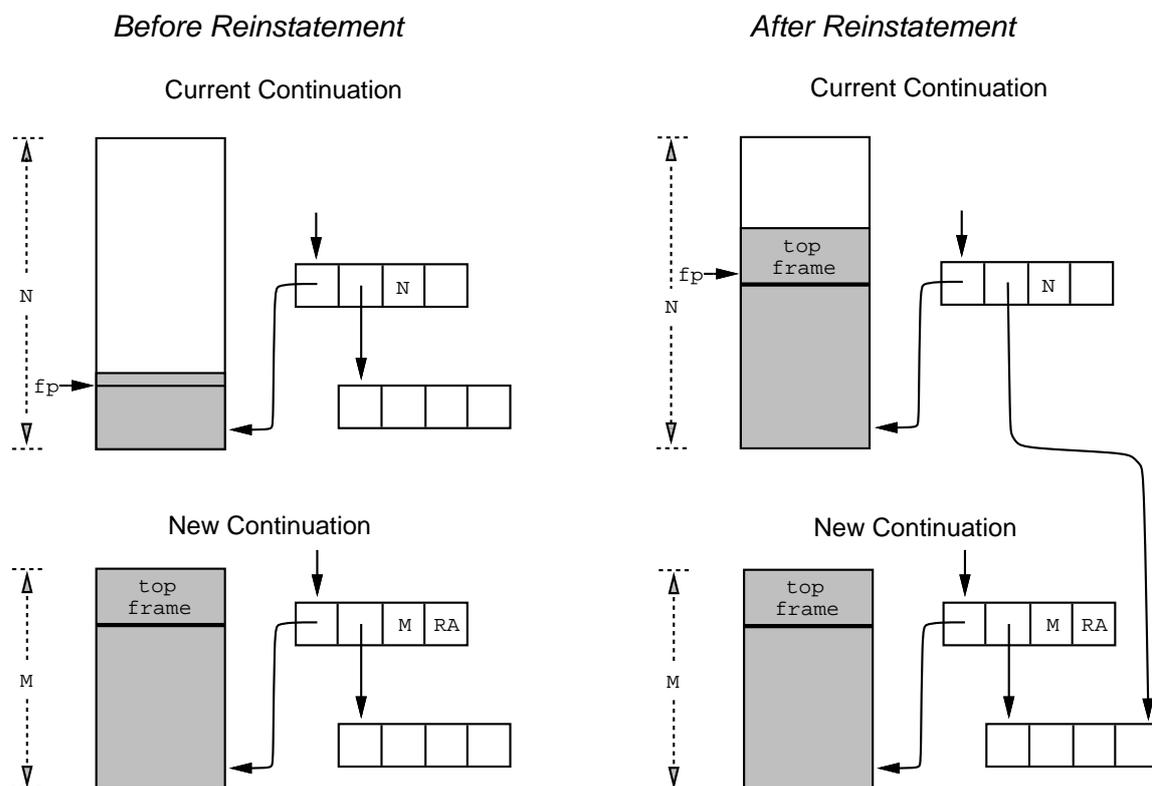
**Figure 6.** When a continuation is reinstated, the contents of the stack segment of the continuation is copied into the current stack segment. If the size of the stack segment is greater than a predetermined limit, the segment is first split into two segments (see Figure 7). If the current stack segment is not large enough to hold the contents of the reinstated stack segment, a new stack segment is allocated.
