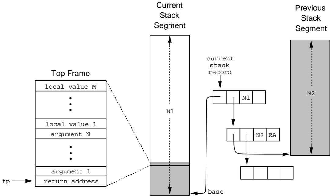
**Figure 3.** The segmented stack model is a simple generalization of the traditional stack model. By implementing the control stack as a linked list of stack segments, continuation operations are bounded by the size of the top segment instead of the size of the entire control stack.
