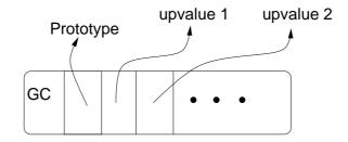
Figure 2: The representation of a closure in Lua.
