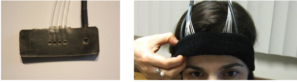
Figure 1. Left: An fNIRS probe with four light source and one light detector. Right: Two fNIRS probes are secured on a participant's forehead using a headband.
