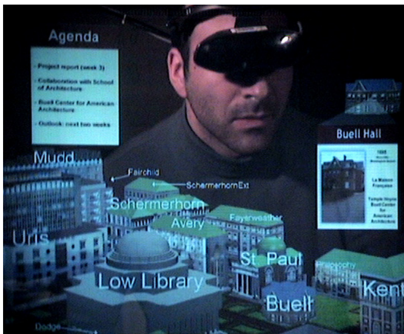
Figure 3. View management applied to the labeling of a virtual campus model and the layout of a meeting agenda and annotated building model, in a collaborative augmented reality system. The layout also automatically ensures that the line of sight is kept clear between the user at the center of the figure and the user from whose view the image is shown. (Photographed through a tracked, see-through, head-worn display.) (From [Bell et al. 2001].)
