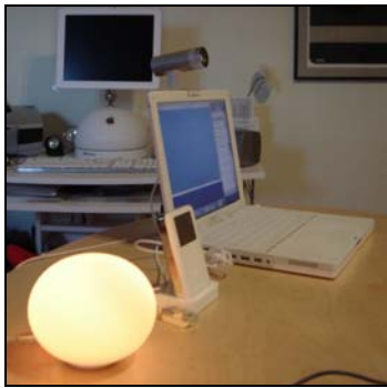
Figure 2. This Ambient Orb (left foreground) allows a user to customize colors associated with trading activity.
