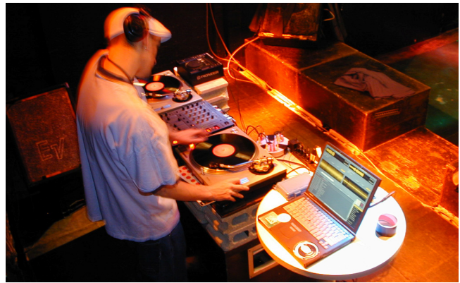
Figure 2 Final Scratch: encoded vinyl for digital music.
