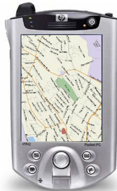
Figure 1. Example of what a Topographic Torch user of sees on-screen. The red dot represents the user’s location in the world.
