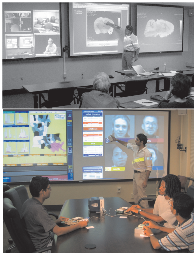
Figure 2. AccessGrid-linked meeting; core tangibles in use (co-located and distributed users collaboratively manipulate a visualization application. Five sets of tangibles (three local, two remote) are used together with data cards to load and save data, manipulate parameters, etc. Most functionality is operational, but image is composited.)
