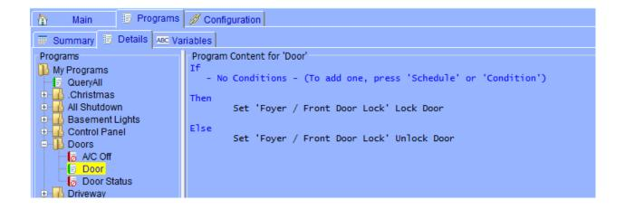
"What that means is that you can map a device called 'Open Door' to the program, allowing you to unlock the door with 'Alexa, turn on Open Door' and lock it with 'Alexa, turn off Open
