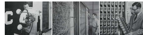
Figure 4.8 Illustration of the Mark 1 perceptron hardware. The photograph on the left shows how the inputs were obtained using a simple camera system in which an input scene, in this case a printed character, was illuminated by powerful lights, and an image focused onto a 20 \times 20 array of cadmium sulphide photoceils, giving a primitive 400 pixel image. The perceptron also had a patch board, shown in the middle photograph, which allowed different configurations of input features to be tried. Often these were wired up at random to demonstrate the ability of the perceptron to learn without the need for precise wiring, in contrast to a modern digital computer. The photograph on the right shows one of the racks of adaptive weights. Each weight was implemented using a rotary variable resistor, also called a potentiometer, driven by an electric motor thereby allowing the value of the weight to be adjusted automatically by the learning algorithm.
