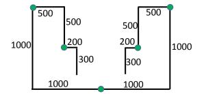
The wire lengths (in DU) are shown on the figure; assume all wires are 4DU wide. The green dots represent inverters.
