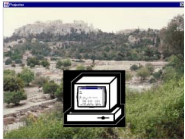
Figure 4. A schematic picture of the Peripheral Border Display prototype. The screen image that is sent to the video projector is shown in the outer window, and the screen image of the regular CRT monitor is shown (here greatly reduced) in the cartoon picture of the CRT in the center.
