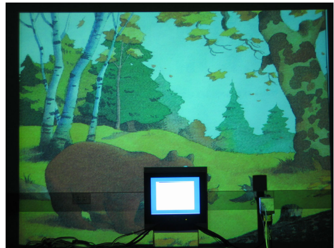
Figure 1: Peripheral Border Display System: The LCD monitor is shown as the light rectangle in the middle of the lower half of the picture. The Polhemus transmitter is shown to the right of the monitor.
