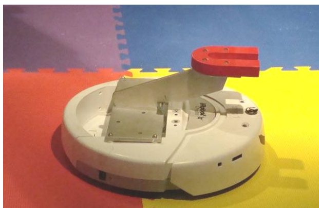
Figure 3. Visitors' programs are sent to an iRobot Create™ robot through a wireless Bluetooth connection. The large red horseshoe magnet on the robot activates the Robot Park sign shown in Figure 2.
