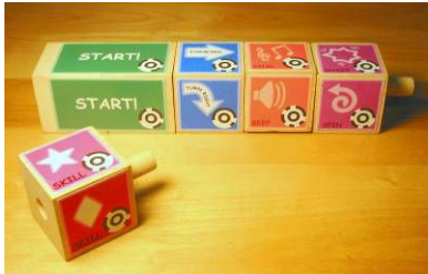
figure 1. Our tangible programming language prototype consists of interlocking wooden cubes with brightly color labels.
