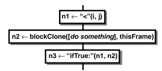
To simplify the example, assume that the SELF compiler is able to infer via type analysis that  $\mathbf{i}$  and  $\mathbf{j}$  are integers. Then the compiler can lookup the definition of < for an integer receiver to find the following method:
