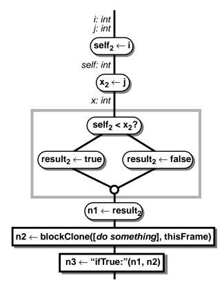
the compiler had delayed the merge until after the **ifTrue**: message, copying all control flow graph nodes between the primitive result and the **ifTrue**: message to get the following graph:
