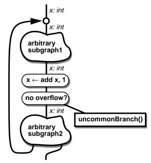
After analyzing the rest of the control flow graph,  $\mathbf{x}$  will be determined to be an integer at the loop tail, which is compatible with the types assumed at the loop head, and so the compiler is done:
