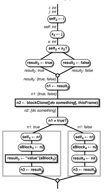
The compiler restarts type analysis, determines that the type of  $aBlock_3$  is a particular cloned block literal, and inlines the block's **value** message down to just the body of the block; the block creation code can then be eliminated since
