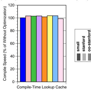
The compile-time message lookup cache speeds compilation by only a few percent. This poor showing is the result of being able to use the cache only within a single compilation and not across calls to the compiler. We are investigating system designs that would support a longer-lived compile-time message lookup cache which we believe could save a significant amount of compile time.
