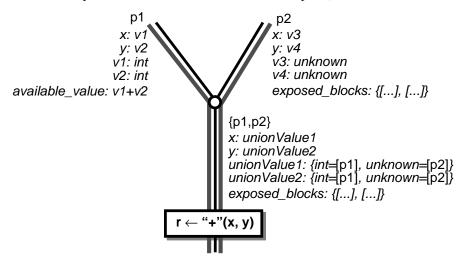
When reaching the + message send, the compiler splits apart the type of  $\mathbf{x}$  to optimize the integer receiver case, producing the following graph:
