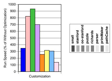
Customization improves performance significantly, enabling these SELF benchmarks to run between 1.4 and 9 times faster. The extra type information provided by customization has been put to good use by the compiler in speeding run-time performance.
