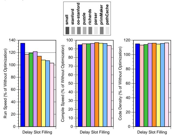
Filling delay slots on the SPARC speeds up the benchmarks by between 5% and 35%, costs little in compile time, and reduces compiled code space requirements by almost 15%.<sup>\*</sup> Given these execution speed and compiled code space benefits, delay slot filling seems to be worth its nominal compile time expense.
