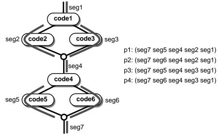
Path segments are concise abstractions of straight-line chunks of the control flow graph. Since straight-line chunks of code are split as a unit, the cost of splitting the nodes in the chunk can be computed once as the nodes are type analyzed and stored in the path segment object. Then to determine the cost of a total split, the compiler can first determine which path segments will get copied as part of a split, and then sum the costs of those path segments.
