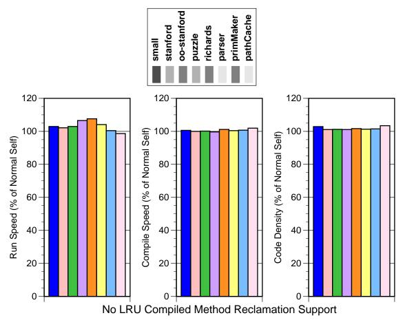
LRU support imposes a run-time cost of up to 8% over a system without this support. This cost is directly proportional to the call frequency of the program being measured. LRU reclamation support takes little additional compile time and little additional compiled code space.
