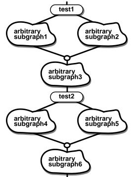
into control flow graphs like the following, with the common-case paths completely separated from the uncommoncase paths, but with each half split apart only when desirable:
