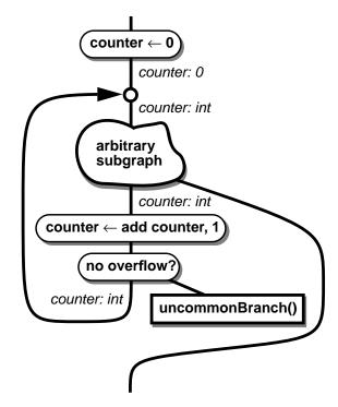
The type at the loop tail is now compatible with the type at the loop head on the first iteration; no additional iterations are needed.
