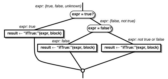
Two copies of the **ifTrue**: message can be inlined away, since their receiver types are both compile-time constants; the third copy remains dynamically-bound since its receiver type is unknown. Control flow re-merges after the type prediction and type casing transformations.
