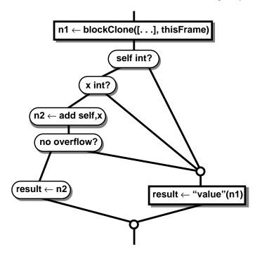
However, since most primitive invocations do not fail, the large majority of the invocations of the primitive do not use the created block. The overhead of creating a block for every primitive invocation, especially ones as simple as integer arithmetic, can quickly bring a system to its knees.
