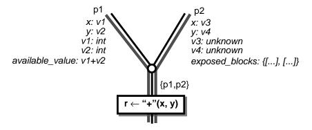
When combining the information after the merge, the compiler creates new union values to represent the bindings for **x** and **y**. Paths are associated with the components of these splittable union types. The compiler must treat the v1+v2 value as no longer available (since it is not available along path p2 and the compiler cannot associate available value
