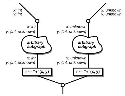
Unfortunately, using the techniques described so far the compiler would not notice that the type of  $\mathbf{y}$  could also be narrowed along the two split branches. This would cause the compiler to insert an unnecessary integer type check for the  $\mathbf{y}$  argument to the **intAdd** primitive that will eventually get inlined as part of the implementation of + for integers.
