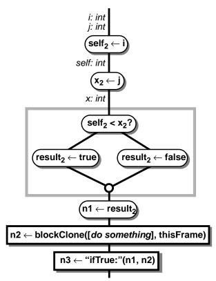
[handle failure] block, since it is no longer needed as a run-time value. These optimizations produce the following control flow graph:
