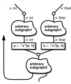
This splitting can create multiple loop heads for a single loop, each loop head for different types. The current SELF compiler's unrolling approach to iteration also creates multiple loop heads each with different types. Consequently, a loop tail may have several loop heads from which to choose when trying to connect to a type-compatible loop head. The compiler tries to find the highest-weight loop head with the most compatible types to connect a loop tail to. If no
