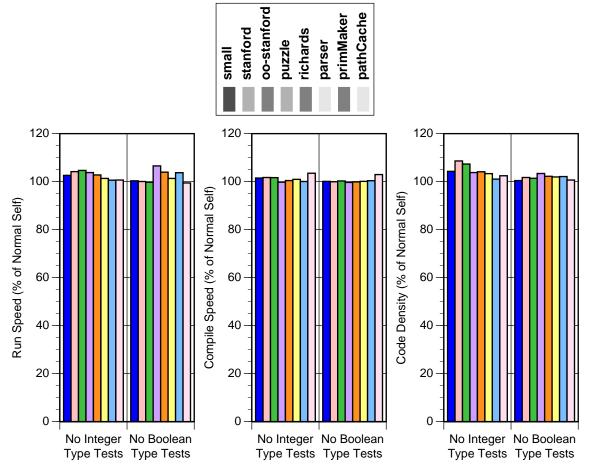
Type tests increase execution time by no more than 10% for these benchmarks, take up little extra compile time, and add no more than 10% additional compiled code space. Type analysis, splitting, and lazy compilation of uncommon cases are largely responsible for the relatively low number of type tests that remain in compiled SELF code.
