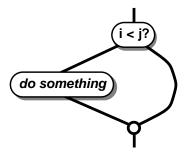
These inefficiencies stem from the control flow merging together after the **intLT** primitive only to be split apart again as part of type casing before the **ifTrue**: message. If the merge after the **intLT** primitive were simply postponed until after the two versions of the **ifTrue**: message, the inefficiencies would disappear, and the SELF compiler would generate the same code as the C compiler. For example, if after inlining the **intLT** primitive to reach the following graph:
