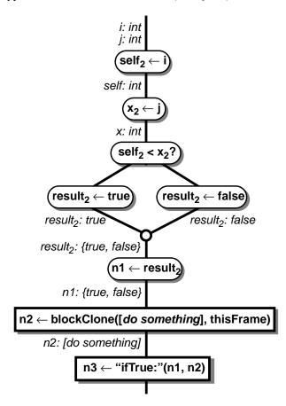
At this point, the compiler could use type-casing to insert a run-time type test to separate the **true** and **false** cases:
