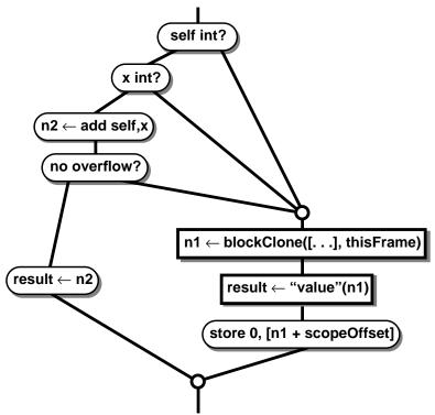
Optimizing away block creations when unnecessary, and deferring remaining block creations until just prior to their uses, is one of the most important optimizations performed by the SELF compiler. As reported in section 14.3, without deferred block creation SELF would run an average of 4 times slower, and more that 10 times slower for programs rife with user-defined control structures such as to:Do: loops.
