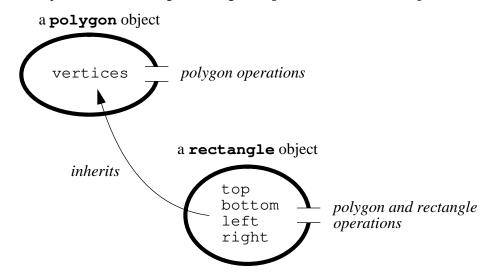
The programmer could make rectangles compatible with polygons by overriding the **vertices** instance variable with a **vertices** method that computed the list of vertices from the four integer instance variables. Unfortunately, in most object-oriented languages overriding an instance variable is not possible, and so **rectangle** cannot inherit directly from **polygon** as pictured. Trellis/Owl and SELF are two notable exceptions to this unfortunate practice.
