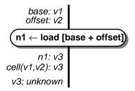
Memory store instructions similarly add a binding from a new cell object addressed by the base and offset of the store instruction to the value bound to the name of the object stored into the addressed memory location.
