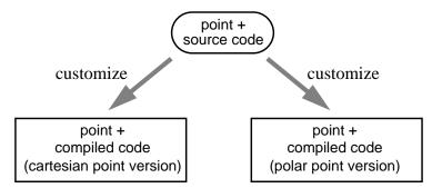
Within each version, the type of **self** is known statically, and the  $\mathbf{x}$  and  $\mathbf{y}$  messages can be statically bound to target methods and inlined.
