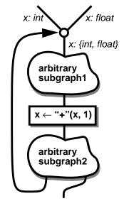
the compiler can split apart the loop head merge node if the variable is sent a message within the loop:
