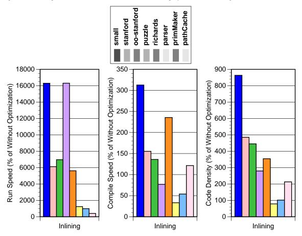
Inlining makes a huge difference in performance. The smaller numeric benchmarks run about two orders of magnitude faster with inlining, and even the larger non-numeric benchmarks run between 4 and 55 times faster with inlining. These results support our contention that aggressive inlining is the key to achieving good performance in pure object-oriented languages.
