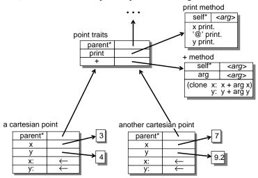
The top-left object labeled **point traits** is inherited by all cartesian point objects. It also contains a parent slot named **parent** containing a reference to another object not shown in this diagram, a slot named **print** and **+** each containing a reference to a method object.
