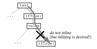
This example is typical of many similar situations in the implementations of common user-defined control structures such as to:Do: and whileTrue:, and some solution must be found in order to achieve good run-time performance.
