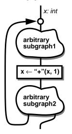
with iterative type analysis the compiler will first assume a set of types for the loop head derived from the loop entry types, in this case that  $\mathbf{x}$  is an integer:
