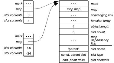
The representation of two cartesian point objects. The objects on the left are the point "instances," containing the values of the  $\mathbf{x}$  and  $\mathbf{y}$  assignable data slots. The object on the right is the shared map for all cartesian points, containing the value of the constant **parent** slot and the offsets of the assignable  $\mathbf{x}$  and  $\mathbf{y}$  slots.
