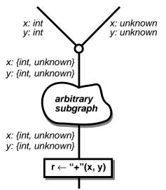
After splitting the + message for the **integer** map type case of  $\mathbf{x}$ , the compiler can alter its type bindings for  $\mathbf{x}$  along the two split branches to get the following split control flow graph:
