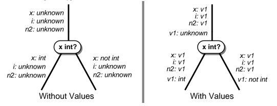
Since many of these type tests occur deeply nested in inlined control structures and operations, the names that are used as part of the test are just local temporary names. Values therefore become critical for communicating this important type information beyond the local scope of the inlined control structure or operation. As shown in section 14.3, without values, SELF would run an average of 50% slower.
