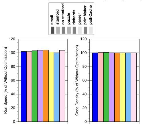
Eliminating the unnecessary arithmetic and memory load instructions saves only a few percent of execution time. If eliminating unnecessary loading of constants were also disabled, the difference in execution speed would be much greater. Virtually no compiled code space is saved by this optimization, indicating that very few arithmetic or memory reference instructions were eliminated in these benchmarks.
