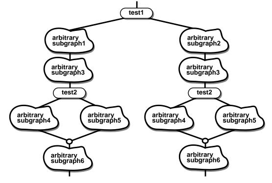
Divided splitting should at most double the size of the control flow graph over straight reluctant splitting instead of exponentially growing the size of the control flow graph as is characteristic of pure eager splitting.
