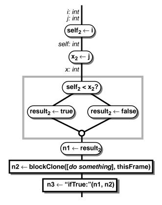
When the compiler reaches the merge node, under eager splitting the compiler does not merge control together but instead pursues each branch independently by duplicating the rest of the control flow graph for each predecessor of the merge:
