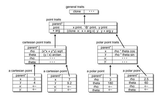
Sending the **x** and **y** messages to (implicit) **self** allows the single **print** method to work for both kinds of points, irrespective of how they actually implement the **x** and **y** messages.
