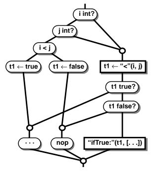
Subsequently, the loads of **true** and **false** may be eliminated as dead assignments, leaving code that is comparable in quality to optimizing C compilers, once the two initial type tests have been executed.
