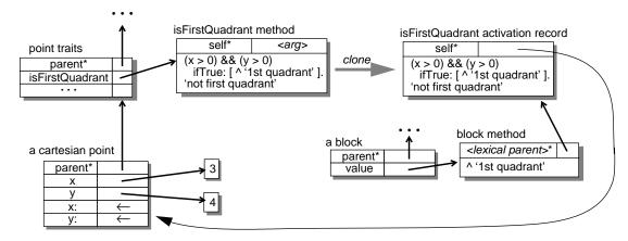
The block object corresponds to the block literal enclosed in square brackets in the **isFirstQuadrant** method. The block's **value** slot refers to a block method object with an anonymous lexical parent slot, which refers to the block's lexically-enclosing activation record object.
