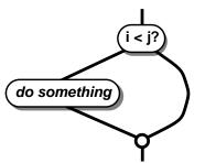
This graph is the same as that produced by the C compiler. To achieve this level of performance and be competitive with traditional languages, the SELF compiler needs some mechanism to postpone merges selectively, to avoid falling back on run-time type casing code. In other words, the SELF compiler needs some *splitting* mechanism.
