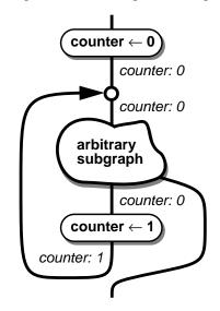
The type of **counter** computed at the loop tail would not be compatible with the type assumed at the loop head, since the type assumed at the loop head would not contain the corresponding type at the loop tail. Consequently, the analysis would be required to iterate with some more general type than the **0** constant type. Since most loops modify some loop counter from its initial constant value, this initial throw-away iteration would be expected for most loop structures.
