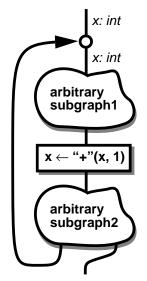
The compiler will then compile the body of the loop under these assumed types. When the compiler reaches the + message, its receiver, **x**, will be determined to be an integer (assuming no other assignments to **x** within the loop), and
