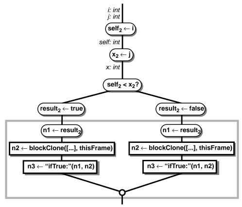
After processing these two branches independently, the compiler reaches the following final control flow graph:
