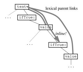
Even this recursion checking is conservative, however. The compiler might be able to inline a recursive call without getting into an infinite loop, if other information available to the compiler makes the processing of the two method invocations somehow different. To illustrate this possibility, consider the **print** method defined for **cons** cells that simply sends **print** to each of the receiver's subcomponents:
