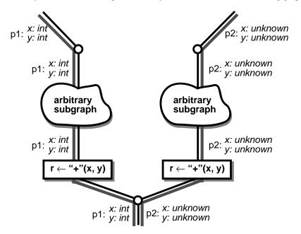
Paths elegantly solve the problem of narrowing the type of  $\mathbf{y}$  appropriately after the split. When the compiler splits off one set of paths from another, in this case splitting off path p1 from path p2, all types associated with the split paths get narrowed implicitly. The type of  $\mathbf{y}$  automatically is narrowed to *int* when p1 is split off from p2, since the type of  $\mathbf{y}$  is associated directly with individual paths, not just with control flow graph nodes.
