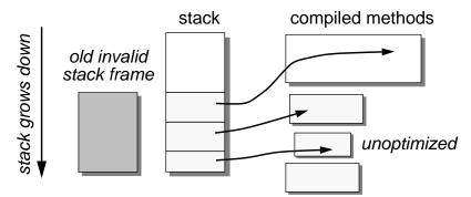
To complete the conversion process, the recompiling routine returns into the appropriate point in the new compiled method for the topmost stack frame. The invalidated compiled method can be flushed from the compiled code cache if the old invalid stack frame is the last activation of this method.<sup>\*</sup>
