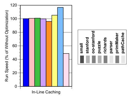
In-line caching makes little impact on the smaller benchmarks, since most sends are inlined in these benchmarks and those that remain are frequently statically-bound to a single target method and so require no in-line caching. The **primMaker** and the **parser** benchmarks benefit more from in-line caching, but not by more than 20%. This result
