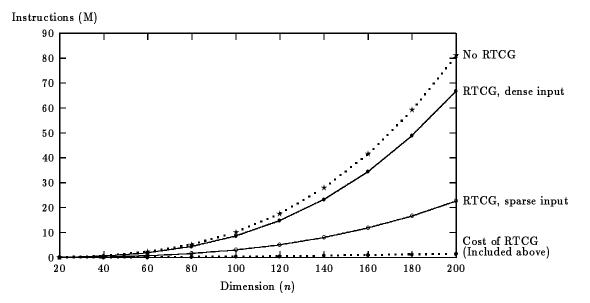
Figure 1: Instructions to multiply two  $n \times n$  matrices
