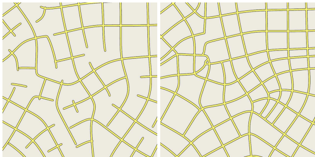
Figure 9: This figure compares a street network in which major and minor hyperstreamlines are traced independently (left) and one using our approach (right). Notice that with our approach the street graph has fewer dangling edges.
