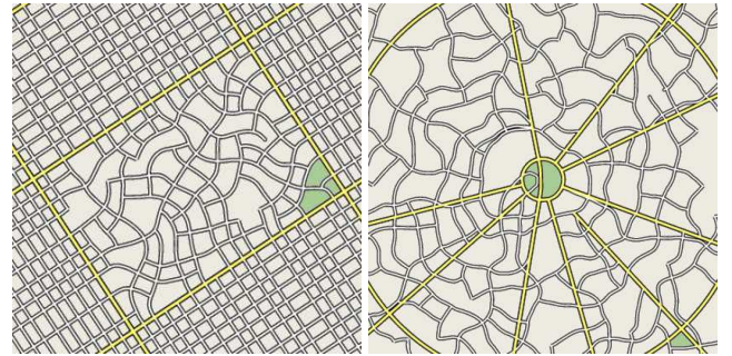
Figure 8: This figure shows a regular major road grid (left) and a radial major road pattern (right) over slightly curved minor roads.
