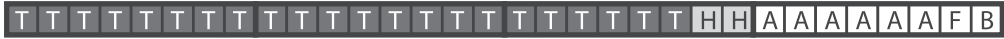
Fig. 3. Jikes RVM object status word bits: thin lock (T), hash state (H), unused bits available (A) for use by the GC, forwarded (F), and busy bits (B).
