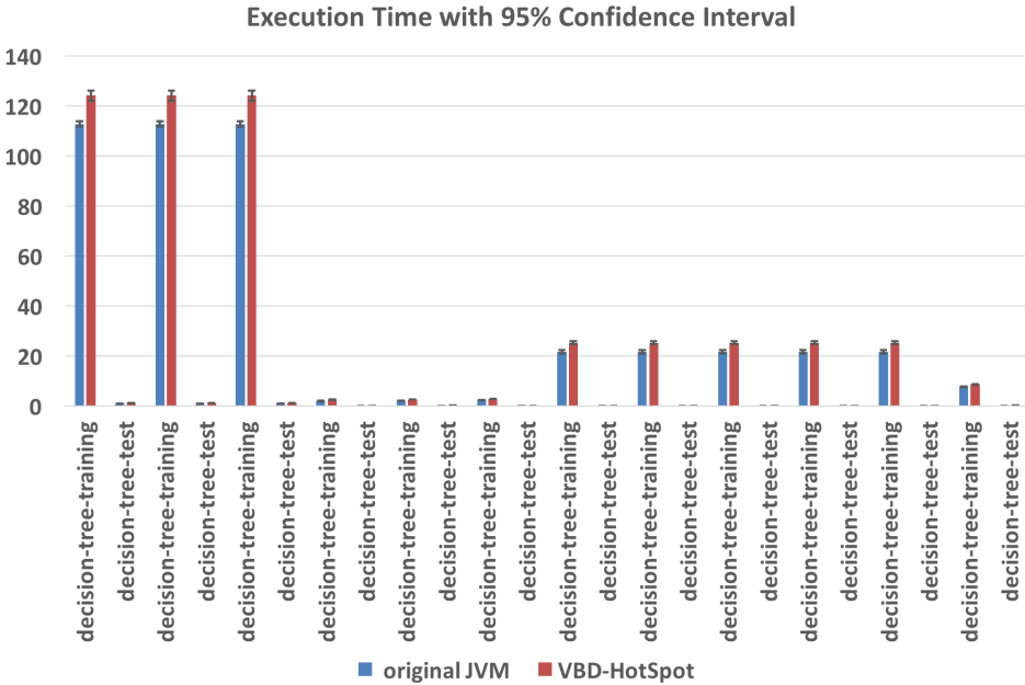
Fig. 8. Average of 10 median execution times in seconds with 95% confidence interval for mllib-tests (part 3 of 4)
